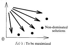
Fig. 10. Search direction of the multi-objective genetic algorithm.
