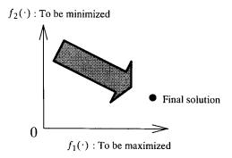
Fig. 9. Search direction of the single-objective genetic algorithm.
