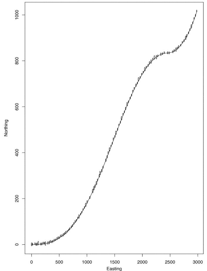
Fig. 8. A 0.9-cut of the fuzzy coordinates produced by a GPS and true trajectory of the vehicle. The distance between a model of the trajectory and the data of the GPS is inherently a fuzzy interval (reproduced from [33]).
