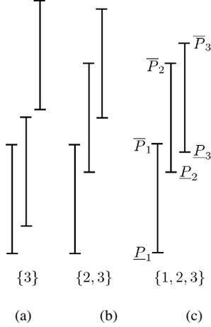
Fig. 1. Example of three possible situations when comparing interval-valued probabilities. (a) The lower bound of  $P_3$  is higher than the upper bounds of  $P_2$  and  $P_3$ , thus the object is assigned to class 3. (b) The lower bound of  $P_3$  is contained in the range of values of  $P_2$  but is higher than  $P_1$ , thus the object can be assigned to classes 2 or 3. (c) The intersection of all ranges is not empty, thus the object can be assigned to classes 1, 2, or 3.
