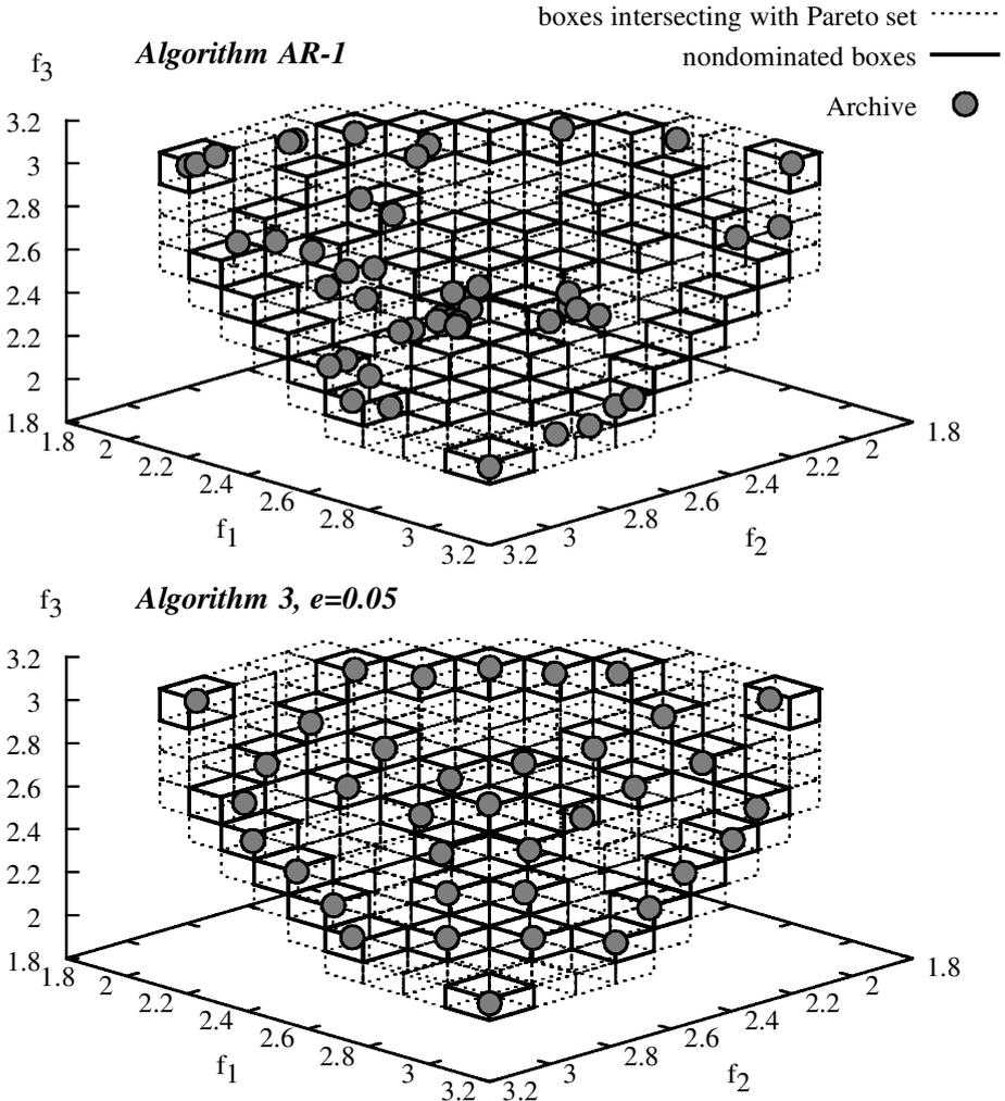
Figure 5: Objective space of MOP (8). The discretization into boxes according to Algorithm 4 is indicated by showing all boxes that intersect with the Pareto set  $F^*$  in dashed lines. The nondominated boxes are drawn in bold lines. The circles correspond to the output  $A$  of different instances of the iterative search algorithm Algorithm 1. For the upper figure, an update function according to AR-1 was used, for the lower figure, the function according to Algorithm 3.
