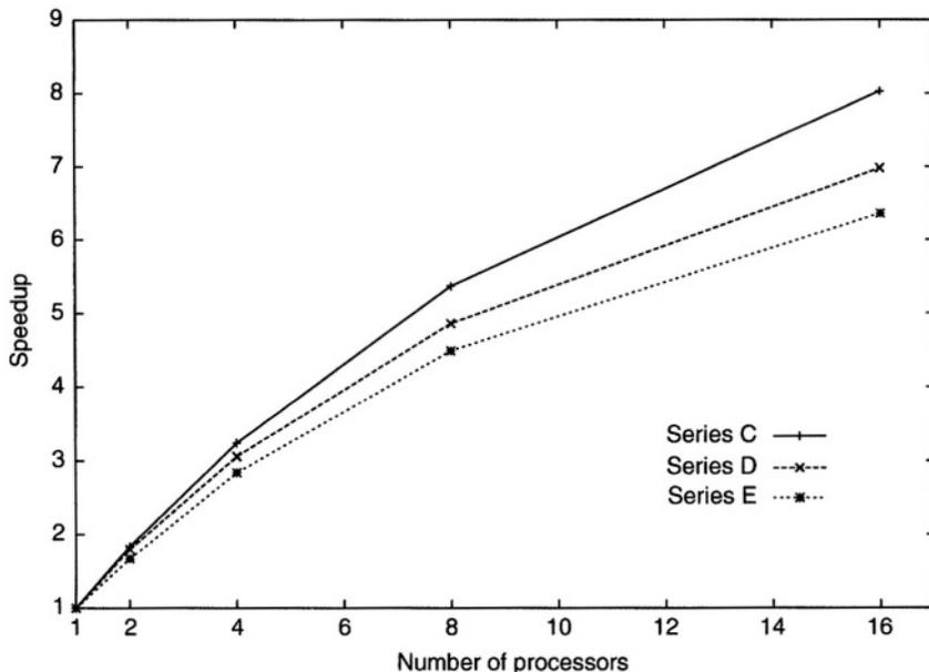
**Figure 8.12.** Average speedups on 2, 4, 8, and 16 processors.
