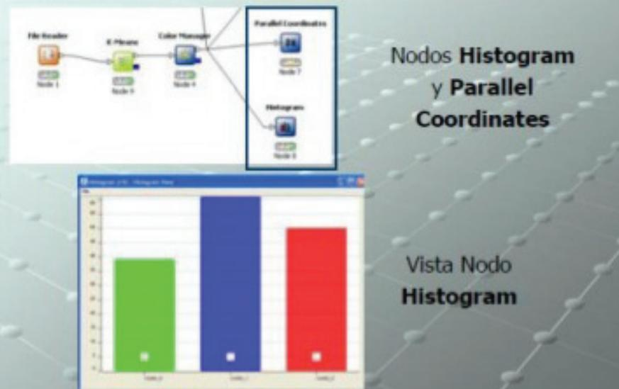
The image shows a KNIME workflow on the left with nodes: File Reader (Node 1), File Reader (Node 2), Color Manager (Node 3), Parallel Coordinates (Node 4), and Histogram (Node 5). A callout box highlights the Parallel Coordinates and Histogram nodes. Below the workflow is a screenshot of a Histogram node's output, showing a bar chart with three bars: green (Node 1), blue (Node 2), and red (Node 3).
