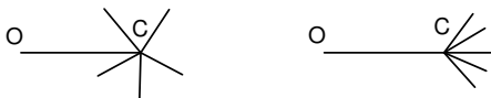
Figure 9. On the left, the normal behavior in which all the space is used to compute the size of each slice. On the right, a modified behavior in which a constraint is applied before computing the size of each slice, allowing us to direct the network in a given way.
