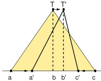
**Fig. 7.** Tuning by changing the basic MF parameters
