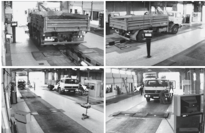
Fig. 3 Whole set of vehicle images used by the system. Two consecutive images are taken as a stereo pair. Each stereo pair shares an image with the previous and the next one: the four images shown form three stereo pairs. As can be seen, using standard matching techniques in order to find corresponding points when measuring the maximum
