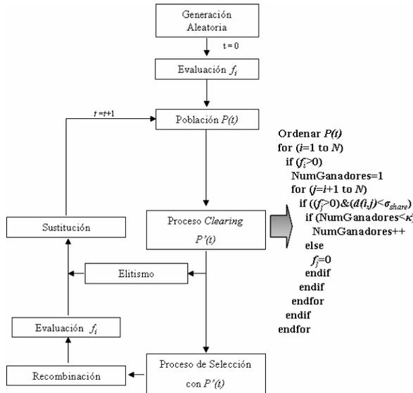
Fig. 1. Algoritmo clearing.
