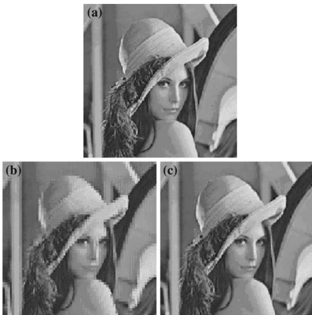
Fig. 4 Comparison of proposed learning algorithm: a Original image; b compressed and reconstructed with SCG only; c Compressed and reconstructed with GA+SCG
