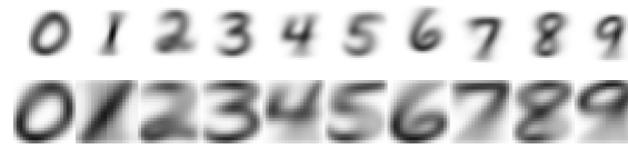
Fig. 3. Average value of 10 images from MNIST, one image per class, before and after applying the centering process.
