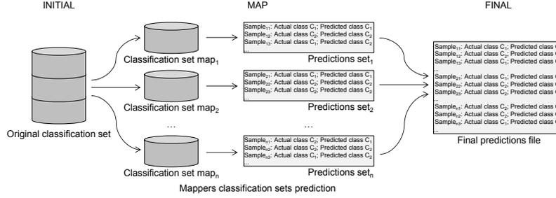
Fig. 3. A flowchart of how the classification of a big data classification set is organized in Chi-FRBCS-BigData
