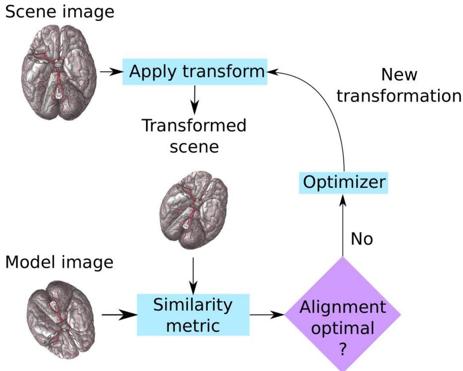
Figure 2. The interactions among the components of a registration technique.
