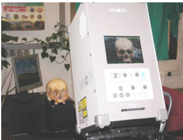
Fig. 1 Acquisition of a skull 3D partial view using the Konica-Minolta laser range scanner of the Physical Anthropology Lab at the University of Granada (Spain)
