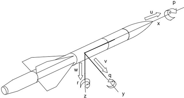
**Fig. 2.** Airframe axes
