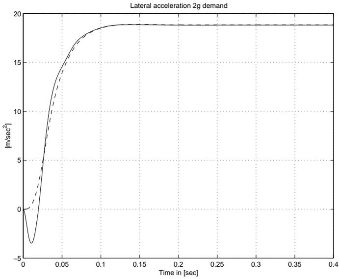
**Fig. 9.** Acceleration Response (b), < 6% steady state error
