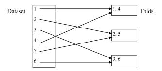
Fig. 3. Assignment of similar instances to different folds. Instances are sorted according to their similarity to the center of the instance space.
