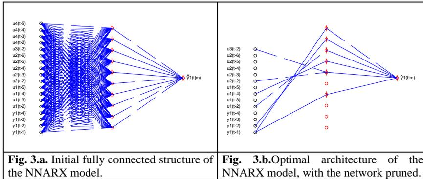
**Fig. 3.** Optimal architecture of the NNARX model, with the network pruned, for the heat flux through exterior walls in the building -output  $y_1(t)$ - (Fig. 3.b.). Positive weights are represented in solid lines, while a dashed line represents a negative weight. A vertical line through the neuron represents a bias. The initial fully connected structure is shown in the Fig. 3.a.
