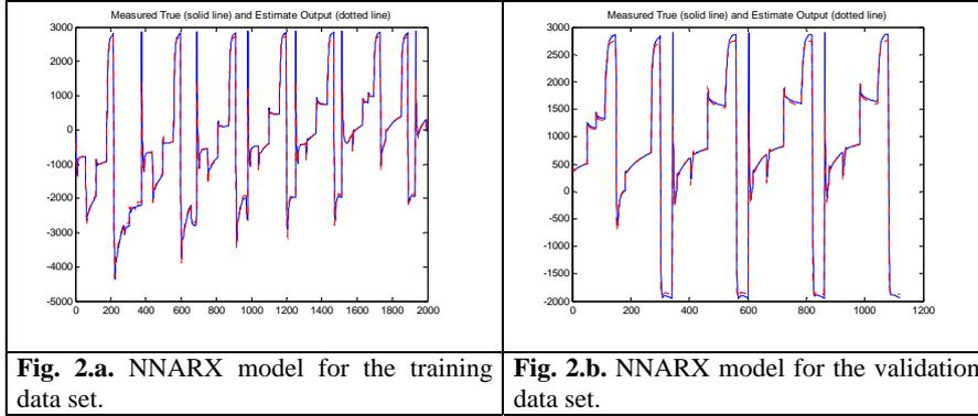
**Fig. 2.** Output response of NNARX model: The actual output (solid line) is graphically presented with one-step-ahead prediction (dotted line). In Fig. 2.a. the real measure can be compared with the estimated data, while in Fig. 2.b. the real measure is compared with the validation data.
