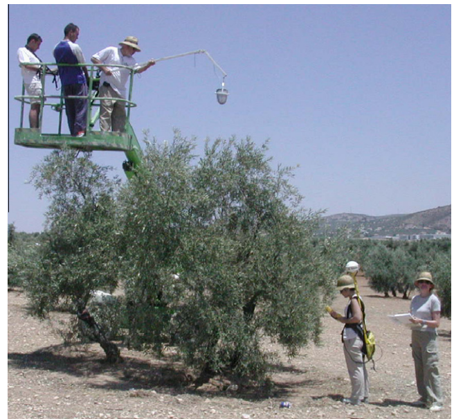
Fig. 2. Measuring olive tree canopy reflectance using a hand-held spectroradiometer with a telescopic pole under sunny conditions. Every olive tree was georeferenced for future remote sensing investigations.
