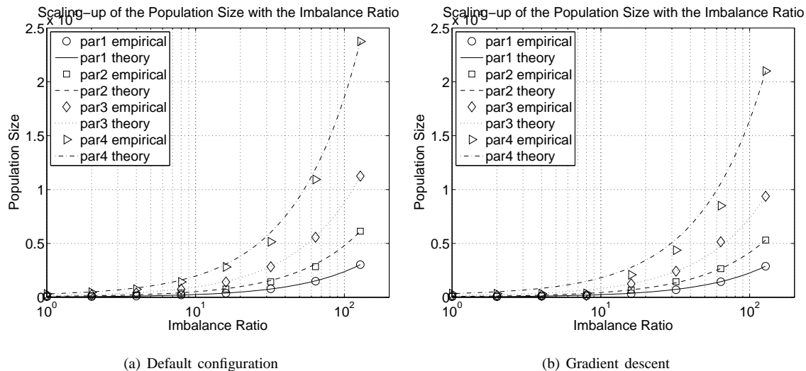
Fig. 5. Scalability of the population size ( N ) with the imbalance ratio ( ir ) in the k -parity problem with k=\{1,2,3,4\} and the default configuration with (a) Widrow-Hoff rule update with adjusted \beta according to ir and (b) Gradient descent parameter's update with \beta = 0.2 . The dots shows the empirical results and lines plot linear increases with ir (according to the theory).
