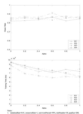
Fig. 10. Effect of mutation reduction rate  $\alpha$  on the performance of IS approaches (test CR and training time) with the wine data.
