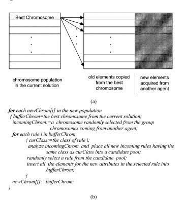
Fig. 7. (a) Illustration for integrating old chromosomes with new elements under IS2. (b) Pseudocode for integrating old chromosomes with new elements under IS2.
