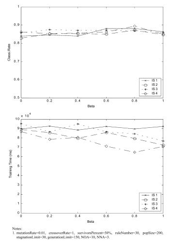
Fig. 11. Effect of crossover reduction rate  $\beta$  on the performance of IS approaches (test CR and training time) with the wine data.
